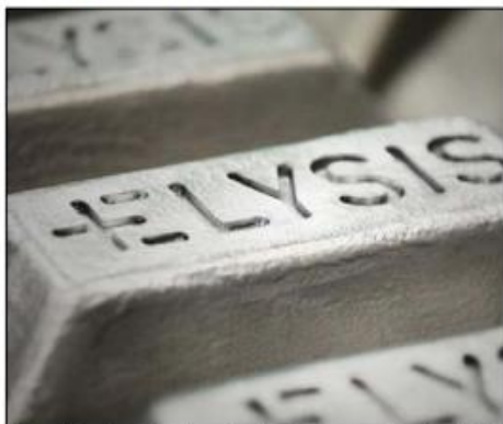
Figure 2. Aluminum ingots produced using the proprietary Elysis technology. (Photo: Elysis.)
