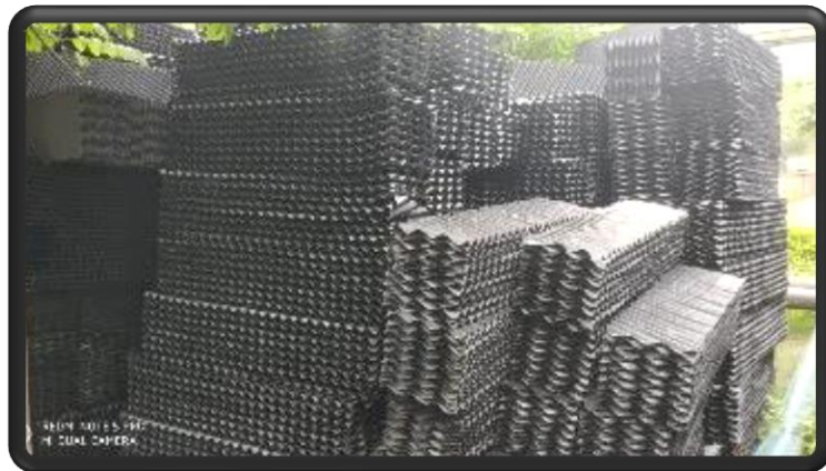
Vacuum improvement by CT fills replacement
