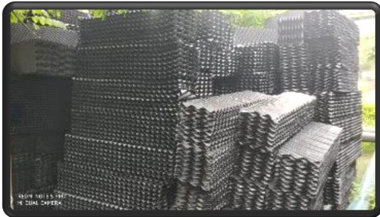
Vacuum improvement by CT fills replacement
