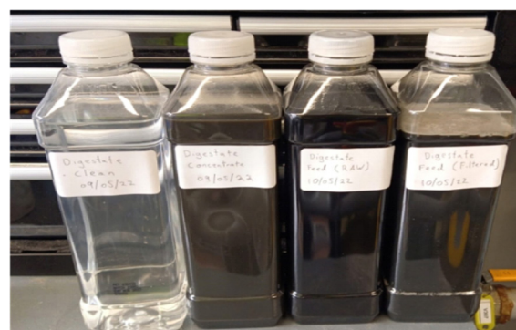
Figure 49: Test samples from anaerobic digester digestate: clean water recovered, concentrate, feed input, raw unfiltered feed
