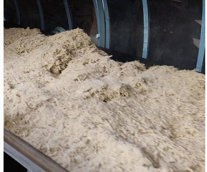
Transport of dry bagasse
