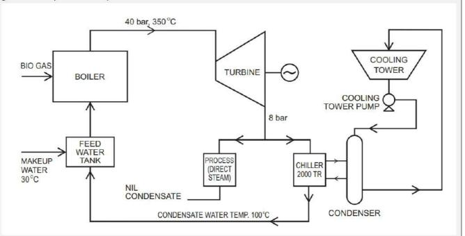
Steam enthalpy at generation pressure and temperature: 720 kcal/kg Enthalpy of back pressure steam : 660 kcal/kg
