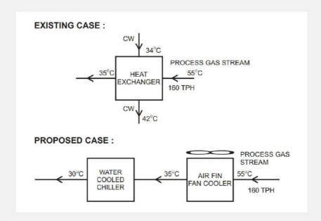
Specific heat of process stream : 0.5 kcal/kg-deg.C
