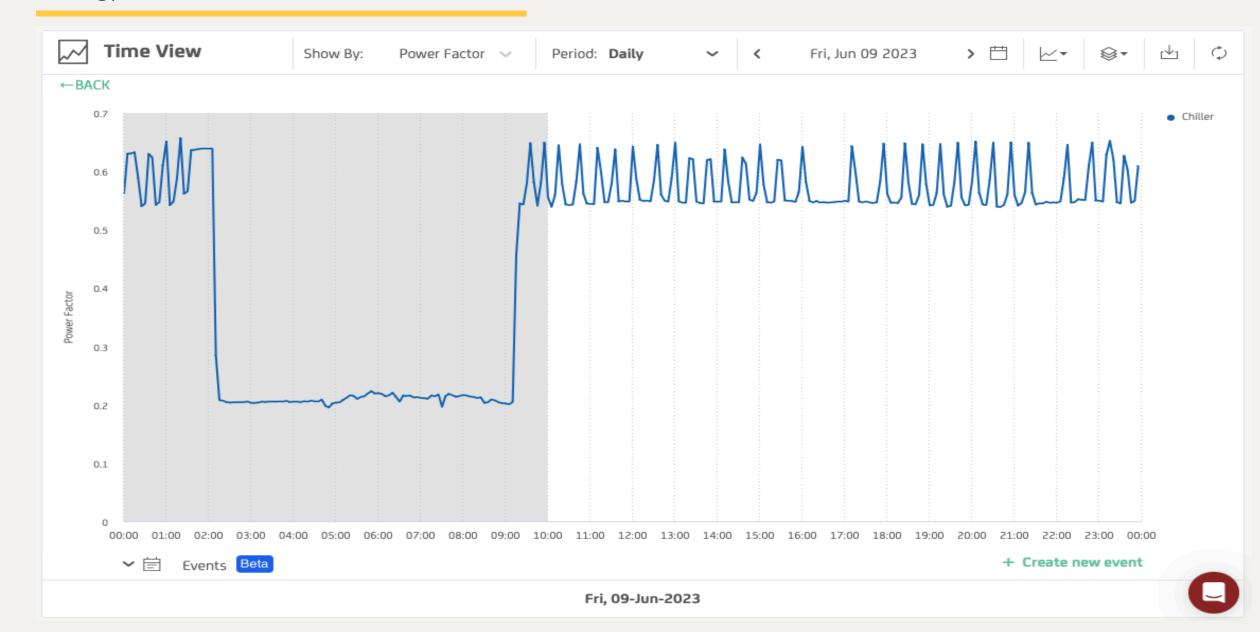
Chiller is consistently operating under 32%, over last 2 months – leads to low power factor & lower efficiency driving higher Energy cost
