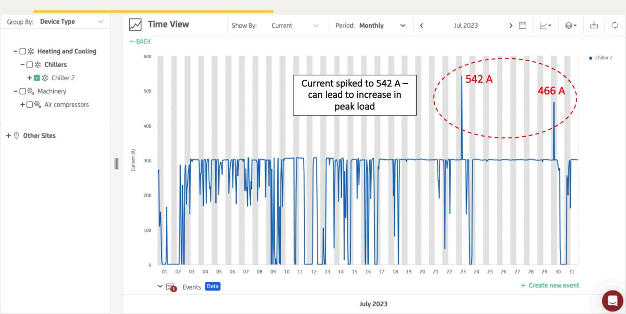
Chiller is consistently operating at a **Power factor in the range of 0.55 to 0.65**, which leads to higher Energy cost and shortens motor life
