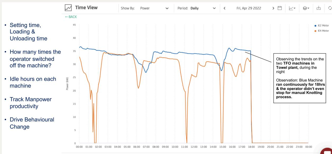
Visibility on how the operator is operating on the machine in Real-time – actual vs. ideal load curve
