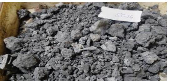
Red mud we are using from Alumina Industries which is very helpful our process to maintain Alkali-Sulphur ratio to avoid jamming & Ring formation at Inlet
