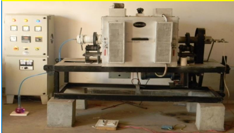
Electrically heated rotary tube furnace at JNARDDC
