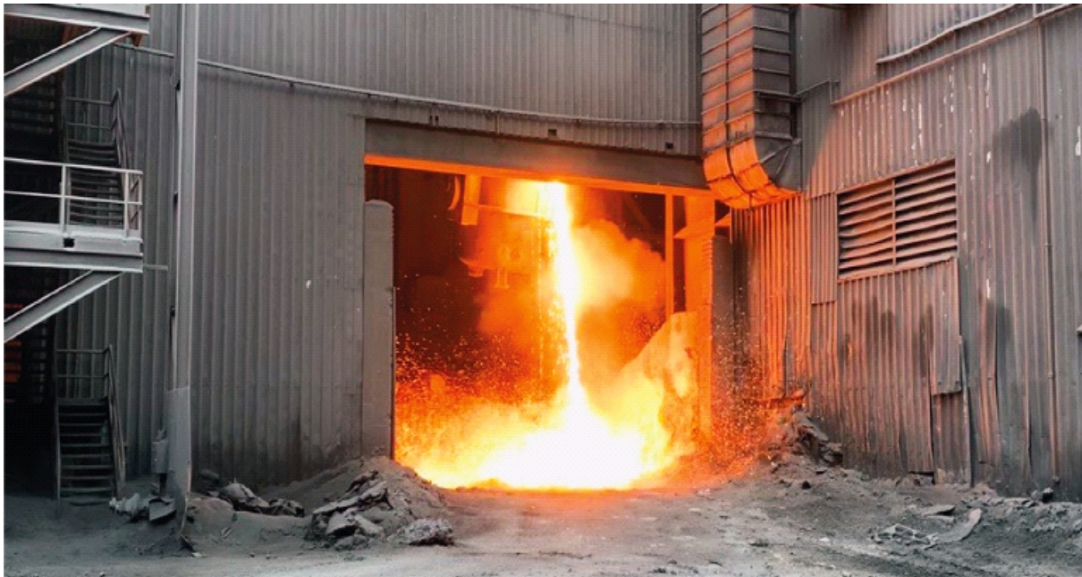
Figure 3: Output of Electric Arc Furnace (EAF) steel recycling process to be cooled to make Portland Cement clinker through Cambridge Electric Cement' process (Source: Cambridge Electric Cement)
