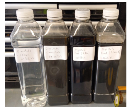
Figure 4: Test samples from anaerobic digester digestate: clean water recovered, concentrate, feed input, raw unfiltered feed
