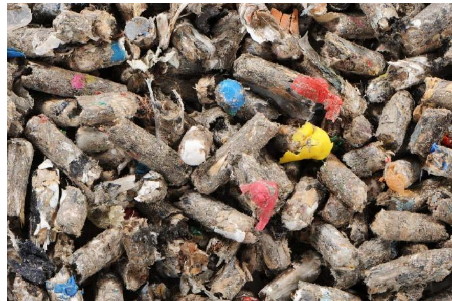
Subcoal is a waste paper/plastic substitute (currently used by Voest Alpine)
