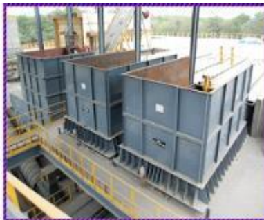
Step – 2 Storage and Feeding Hoppers
