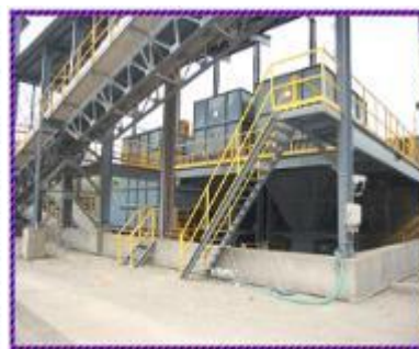
Step – 3 Storage and Feeding Hoppers
