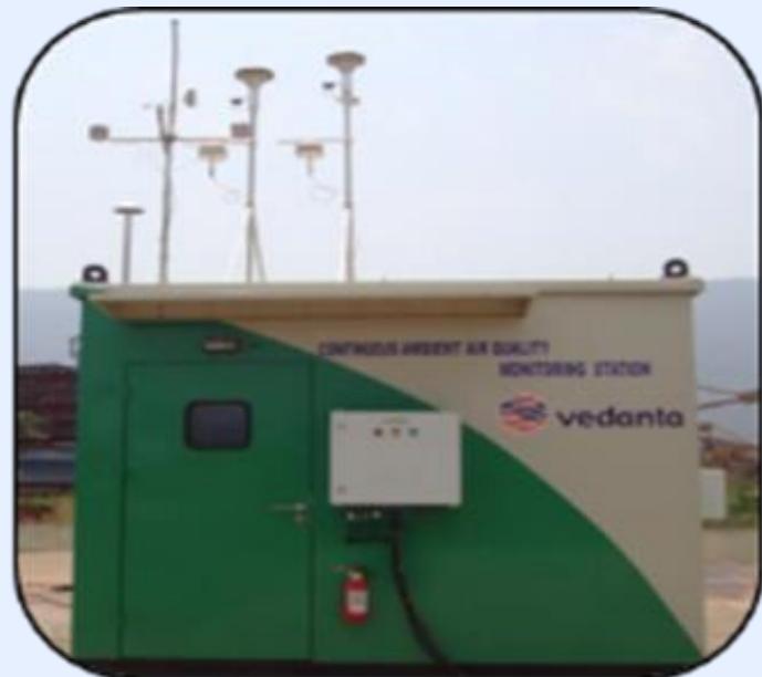
Continuous Ambient Air Quality Monitoring Station (CAAQMS)
